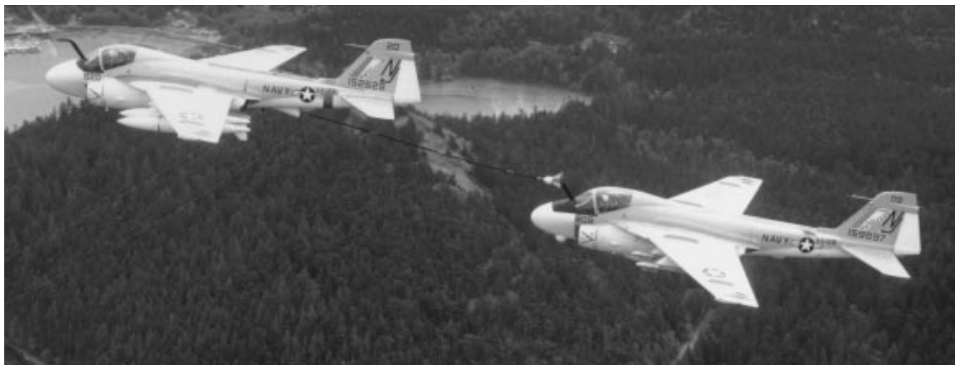
Squadron A-6E Intruders conducting aerial refueling, 1982.
